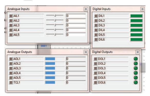
Analog Inputs can be manipulated by entering a value in the field next to them. Digital Inputs can be switched on and off.
