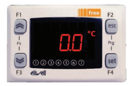
This window can be controlled just like a physical PLC. Buttons can be activated by clicking on them. To activate F1 and F3 simultaneously click on F5 between the buttons.
