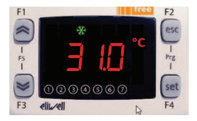
Change Analog Input 1 now back to a Value smaller than Setpoint and the Digital Output and on Screen Cooling display will turn Off.
