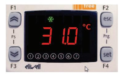
When Analog Input 1 reaches a value smaller than Setpoint, the Digital Output1 and on Screen Cooling display will turn Off again.
