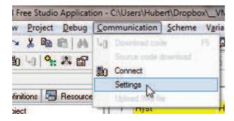
Activate the Protocol that you are using for communicant either Modbus or EwDMI.
