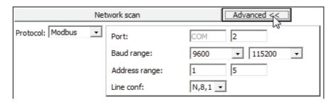
Port: You need to select the Com port where your converter is connected to Baud range: Search will run through all selected Baud ranges in order to search for a device Address range: Search will run through all selected Address ranges in order to search for a device Line conf: Default in SMART is E,8,1 but N,8,1 is also a very commonly used configuration.
