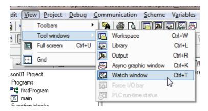
To monitor a variable in the Watch window either click on Variable and drag it while holding mouse button into the Watch window, or click on variable and press F8.
