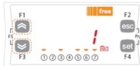
Use the UP and DOWN keys to change the value if necessary. To confirm the value press the set key. To exit press Esc
