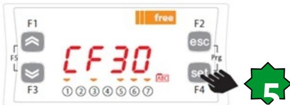
The first parameter shown is CF30. To view the value of the parameter press the set key.
