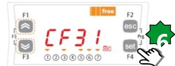
Use the UP and DOWN keys to scroll the other parameters and repeat the procedure to view the values and - if necessary - edit them.
