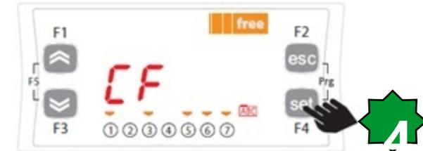
The first folder shown is the CF configuration folder. Press the set key to view the folder parameters.
