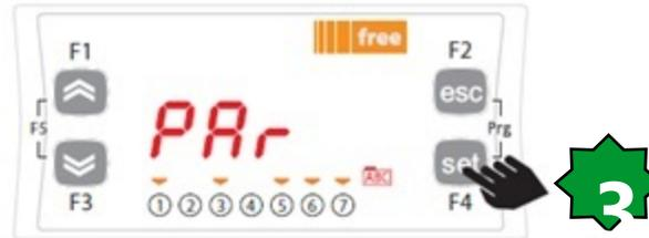
The parameters menu PAr contains all controller folders. Press the set key to view folders.
