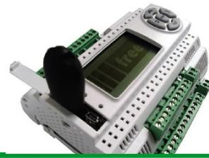
The upload process starts when the pen drive is plugged and can be monitored through the led status which, during the upload process, are controlled directly by Evolution bios.
