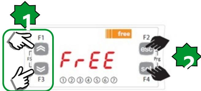
To view the parameter menu, press the Esc and Set keys at the same time. This will open the PAr menu.
